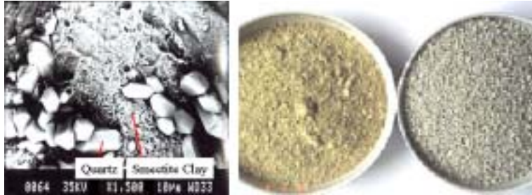
Figure 5. ESEM (Electronic scanning electron microscope) photograph showing artificial minerals (left) and crushed mineral grain (right).
