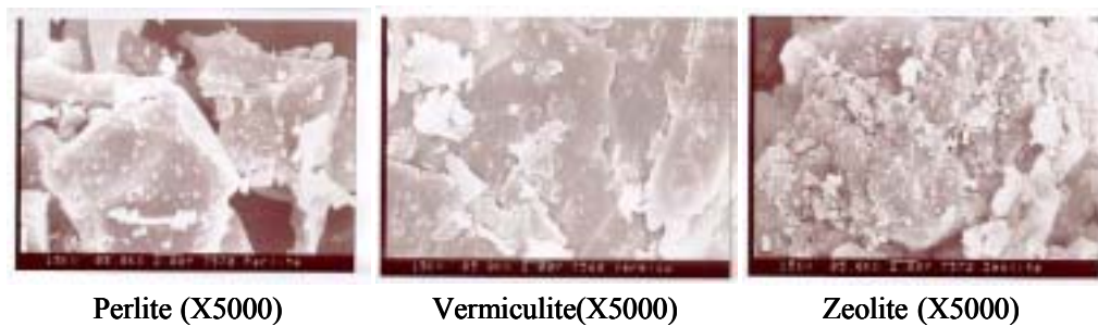
Figure 33. Pictures taken by ESEM for the minerals particles passed through 0.25 mm sieve.
