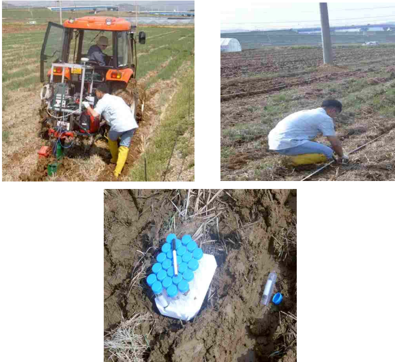
Fig. 2-17 Collection of the soil samples in field
