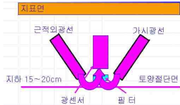
Fig. 2-3 Concept design of the developed soil organic sensor
