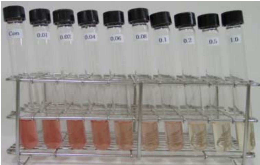
Fig. 66. Results of Rapid Fungicide Residues Assay using color formation with CMB03 test ( mancozeb : 0 - 1.0 ppm )
