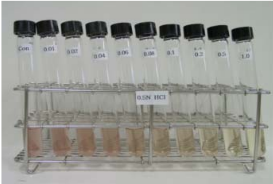
Fig. 35. TTC test with 0.5N HCl of stop solution in various concentration of mancozeb
