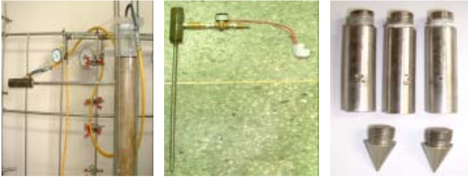
Figure 5-19. Pictures showing the components to test the fracture of soil at laboratory scale.
