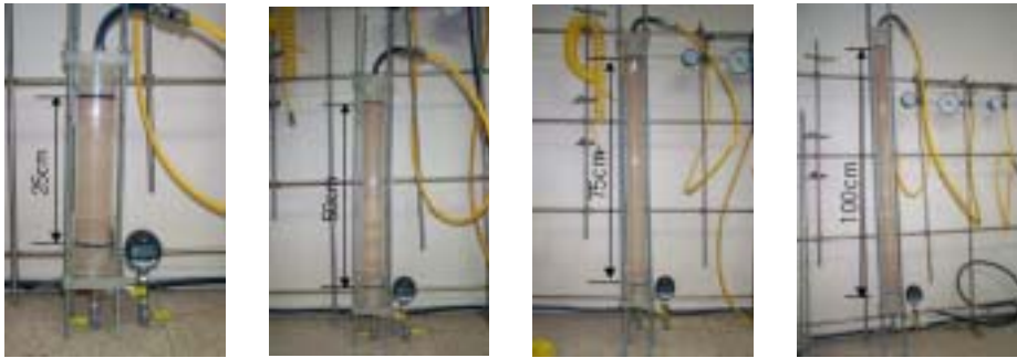
Figure 5-21. Soil column used to measure the air permeability under the saturated condition.
