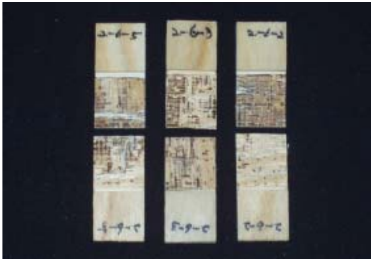
Figure 1.5. Specimens after tension shear test.
