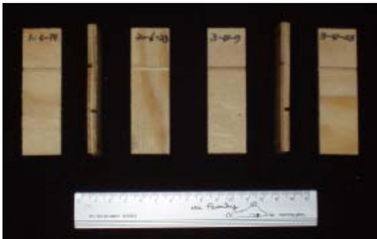
Figure 1.4 Tension shear strength specimens used in this study.
