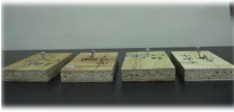
Figure 4.1. Wood screw withdrawal failures for Com-Ply specimen.
