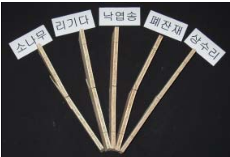
Figure 1.9. Specimens failures after static bending test.
