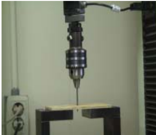
Figure 3.1. Testing arrangement for nail push through the thickness of specimen.
