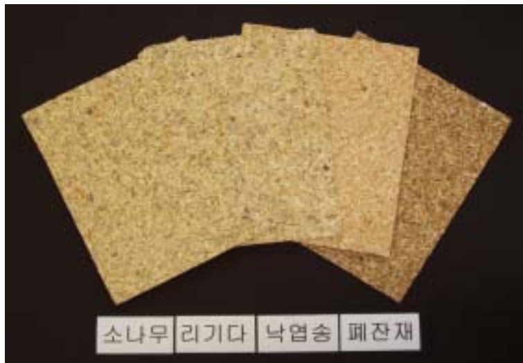
Figure 1.2. Particleboard made from thinning logs in this study.
