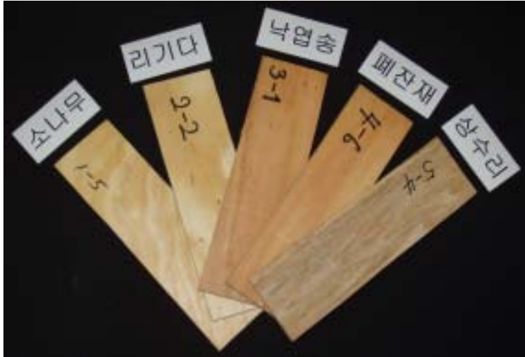
Figure 1.7 Com-Ply made in this study.
