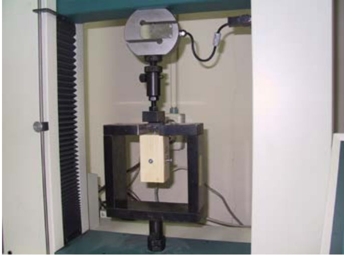
Figure 5.1. Testing arrangement for wood screw withdrawal test.
