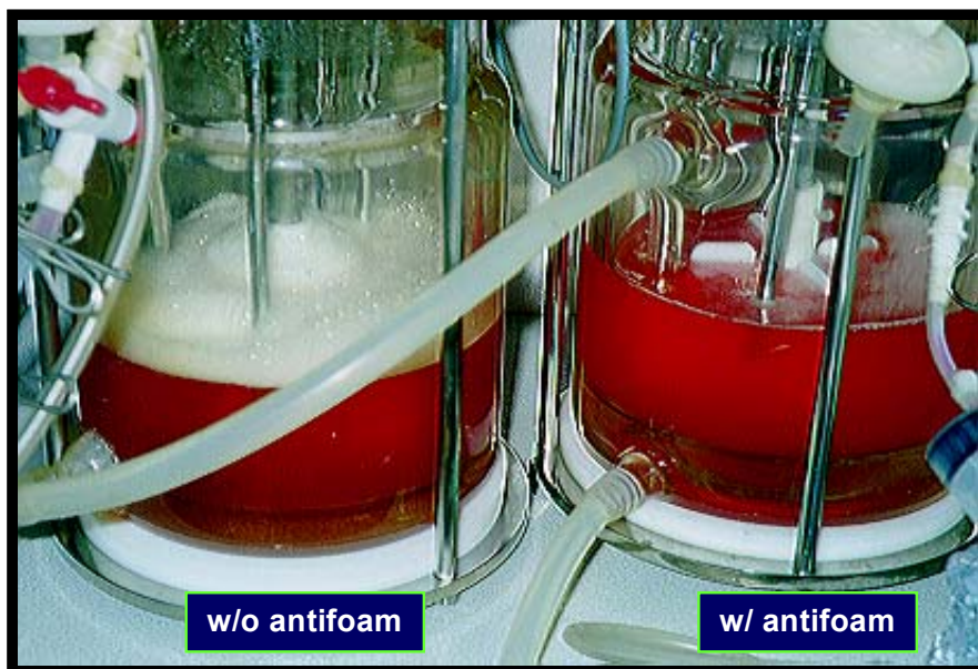
Fig 3.35 Formation of forms when air was supplied continuously by the microsparger in 2 liter bioreactor system (Left: when antifoam agent was not supplemented; Right: when antifoam agent was supplemented).
