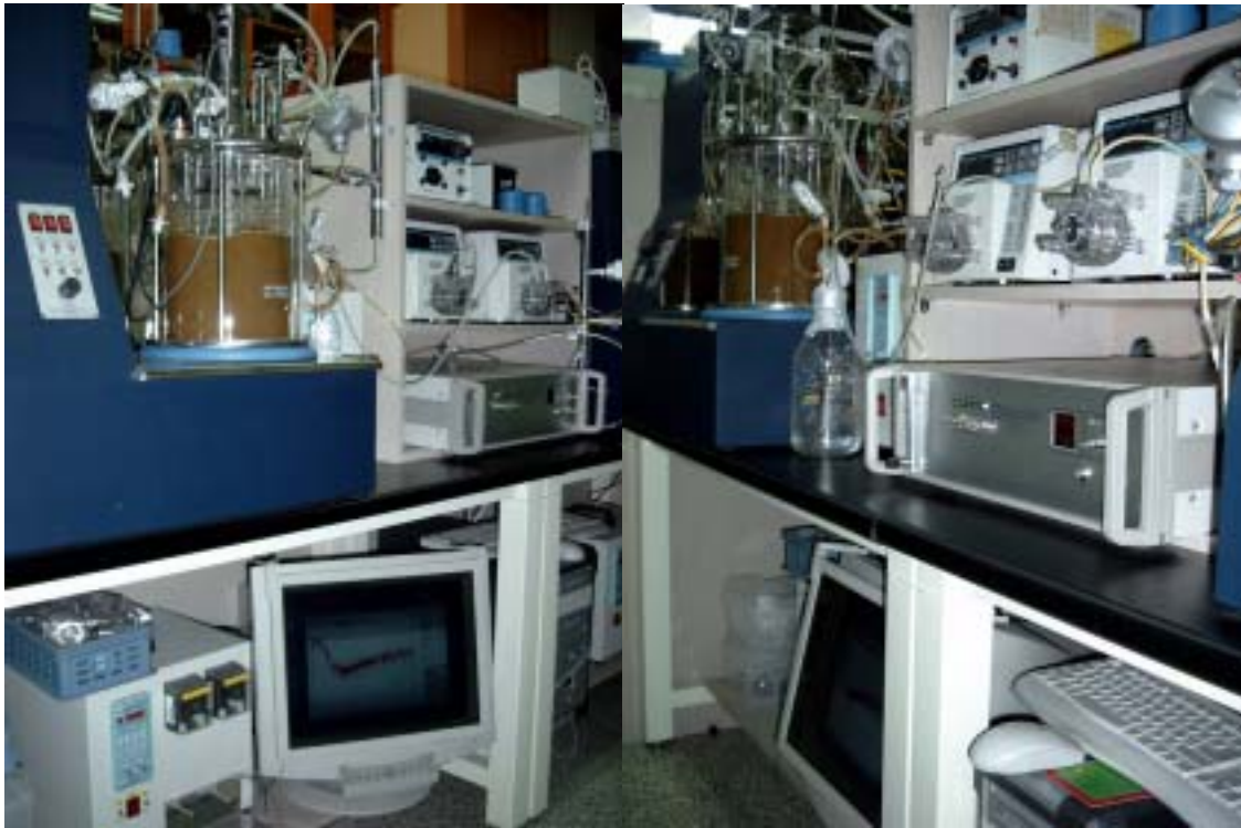
Fig 3. 38 Photograph of on-line measurement system for the estimation of cell cultivation parameters.
