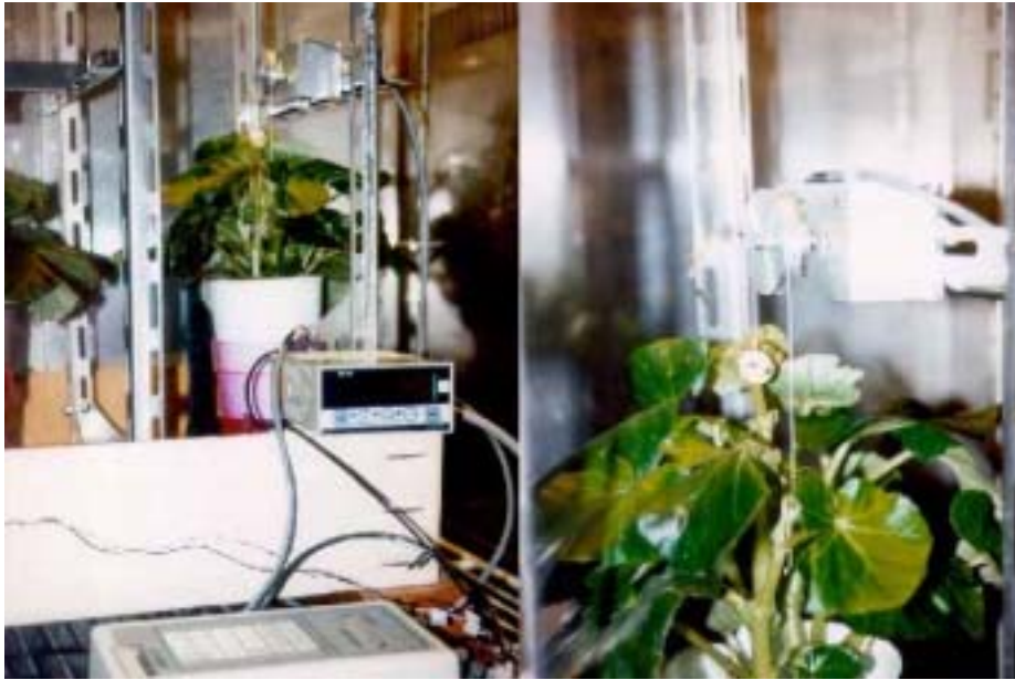
Fig. 2. Diurnal growth measuring system used in this experiment (left: rotary motion sensor, right: pulley).
