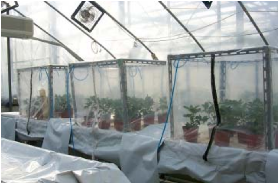
Fig. 1.25. CO 2 injection system used during the experiment.
