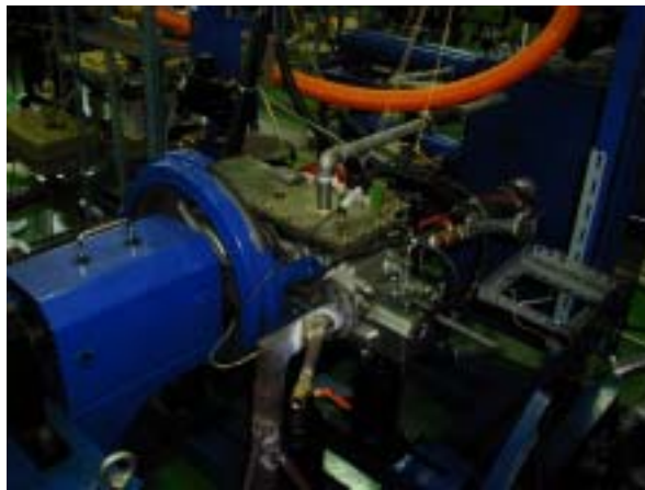
Fig. 3-3 Experimental apparatus of 1 cylinder engine(ND130)
