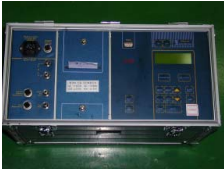
Fig. 3-7 Experimental apparatus(Exhaust gas analyzer)
