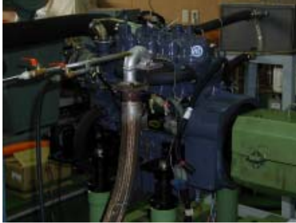
Fig. 3-4 Experimental apparatus of 4 cylinder engine(TD1700)
