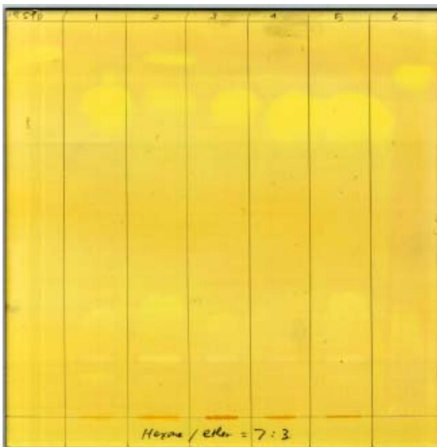
Fig. 1. TLC chromatogram of total lipids extracted with chloroform/methanol(2:1) from various fish species containing wax esters using solvent system of hexane/diethyl ether (7:3, v/v). The chromatogram shows bands of Wax esters standard, Spanish Mackerel, Pollack, Horse Mackerel, Mackerel, Atka Mackerel, and Myctophid from the left.
