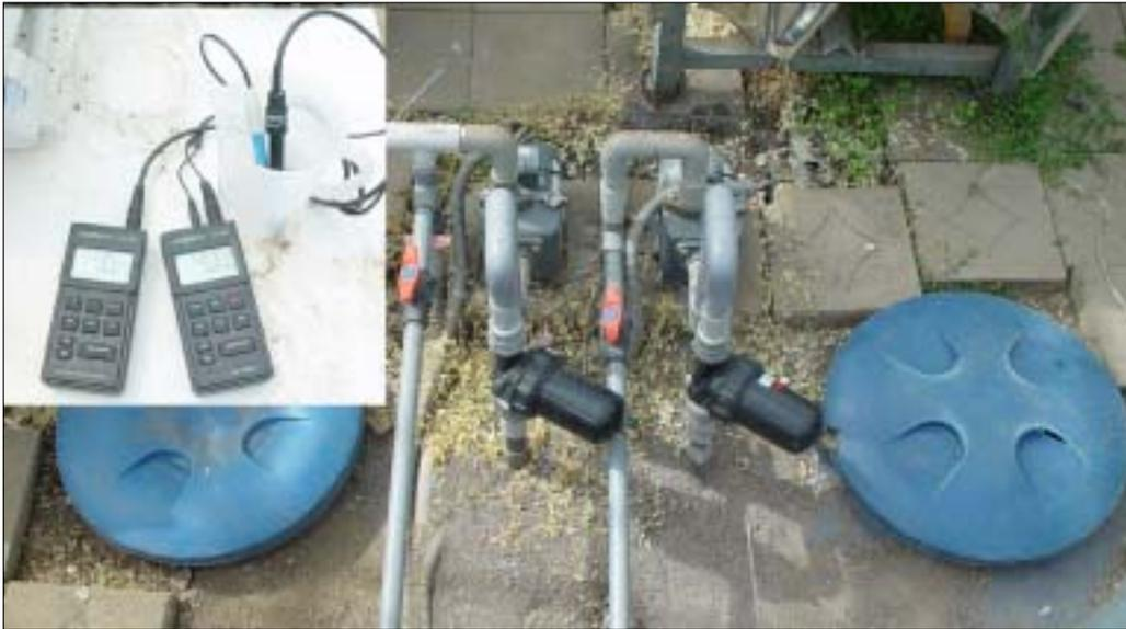
Fig. 1. Equipments for measure of pH and EC and for the supply of pump, filter and nutrient solution reservoir of aeroponic system for seed potato production used in the development of the wick hydroponic system.
