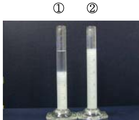
Fig. 16. Comparison of dispersion property of freeze-dried rice powder (5% w/v) gelatinized by conventional and ohmic heating.
