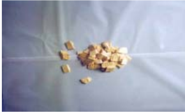
Fig. 2-19. Photographic woodchip for sewage treatment.
