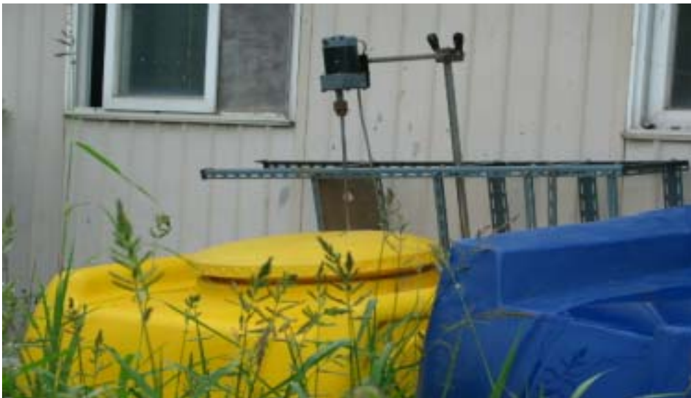
Figure 4-5. Mixed bioreactor(1 m 3 ) made from FRP
