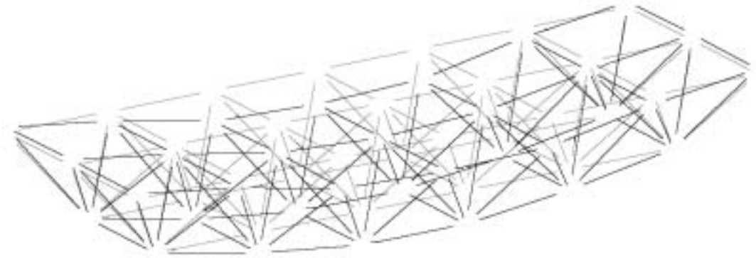
Fig. 7-34. Concept drawing of deflected wood space truss after loading
