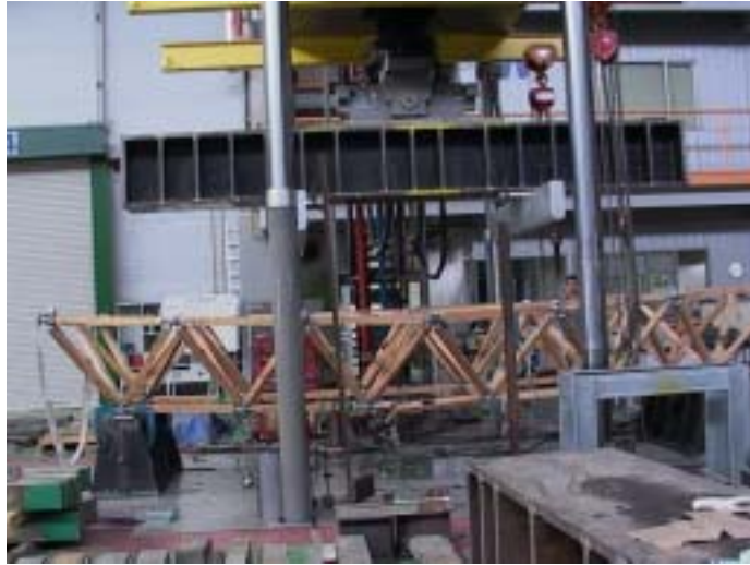
Fig. 7-19. Full-scale specimen tested for wood space truss
