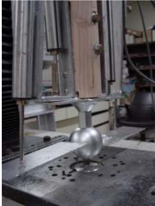
Fig. 7-7. Tension tests of connectors for wood space trusses
