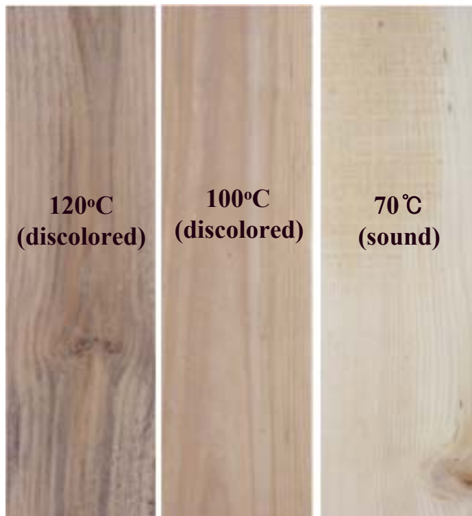
Fig. 3-19. Comparison of the extent of surface discoloration at three drying temperatures in Korean white pine.
