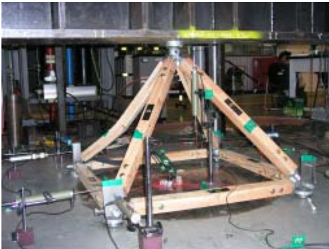
Fig. 7-12. Deformed unit wood space truss after test
