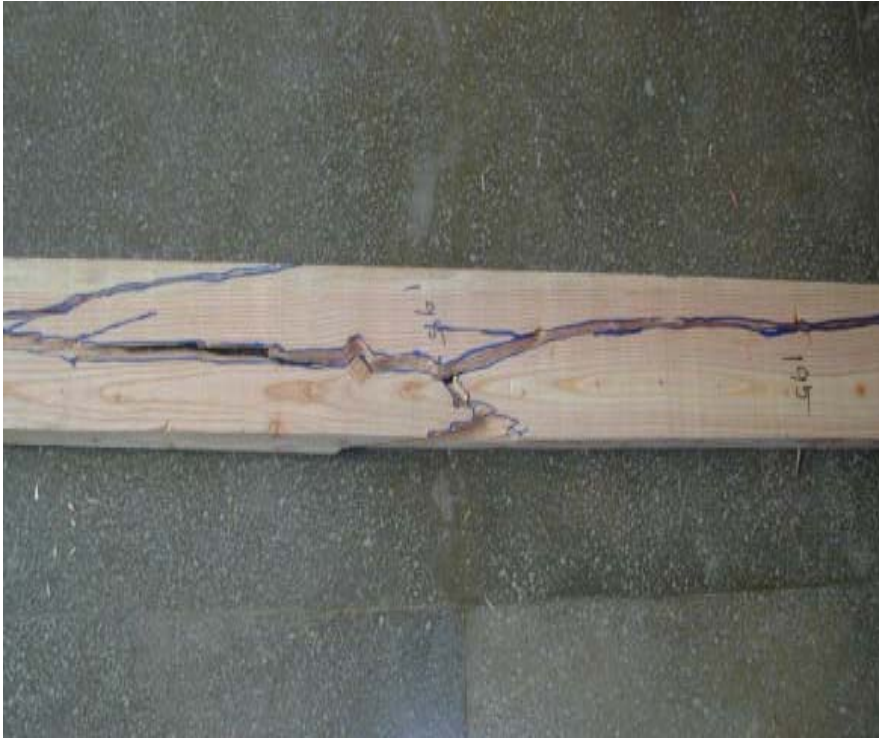
Fig. 6-31. Example of failure mode for bending test (simple tension).
