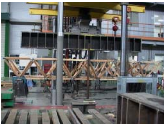
Fig. 7-18. Full-scale flexure testing of wood space truss
