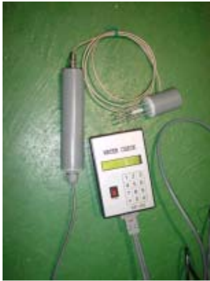
Fig. 3-4. Moisture content sensor with three pins.
