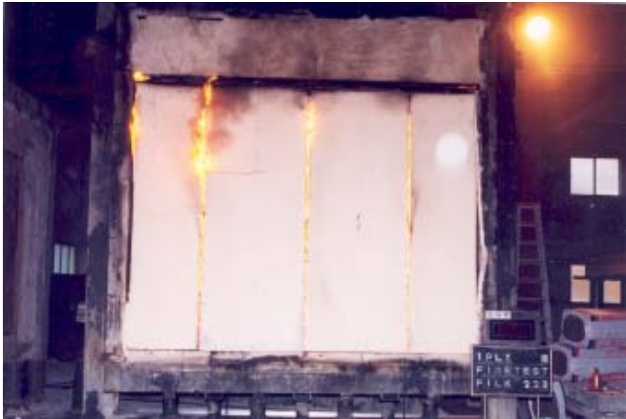
Fig. 4-17. Fire test set up for wall structure
