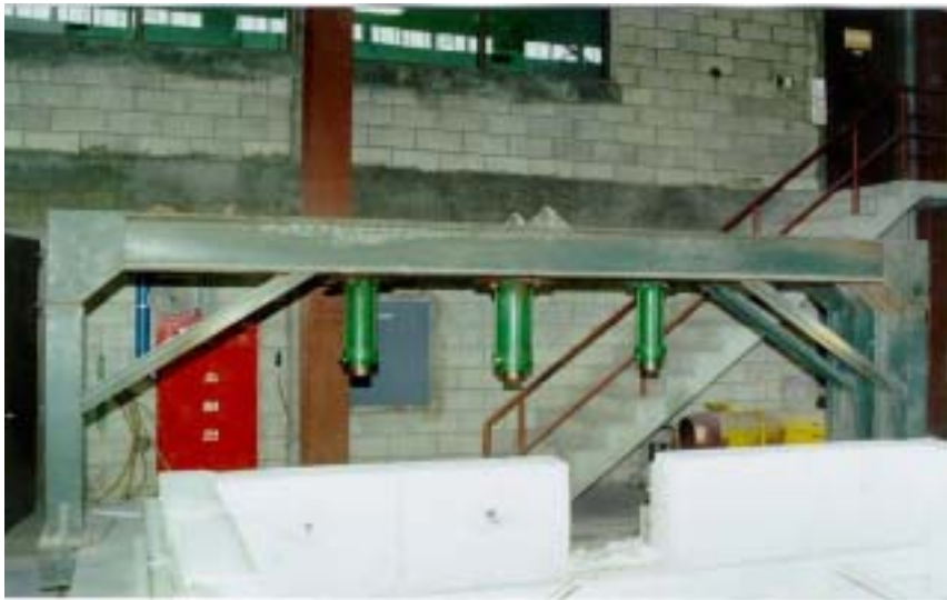
Fig. 4-14 Loading system of horizontal furnace
