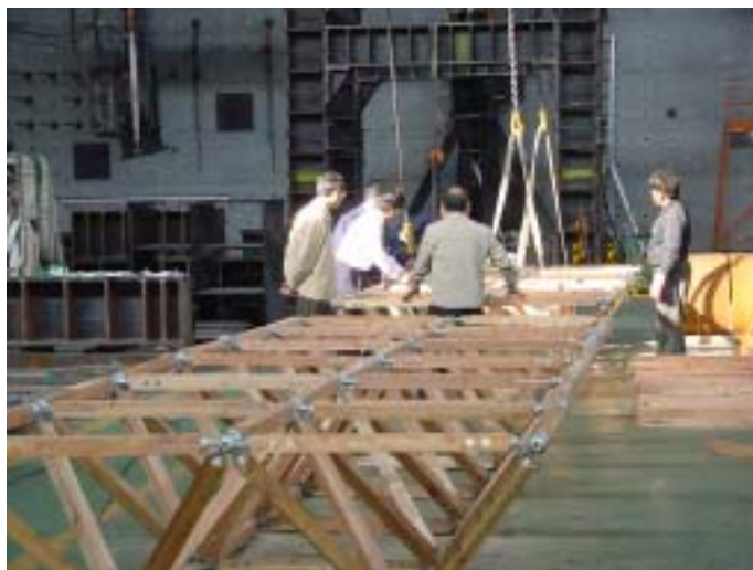
Fig. 7-17. Full-scale test specimen of wood space truss
