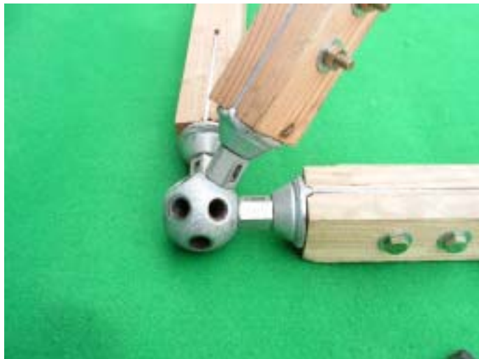
Fig. 7-5. Connector developed for wood space trusses
