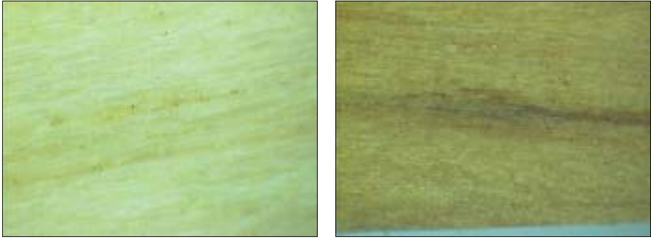
Fig. 3-18. Non-discolored(sound) surface of Korean white pine(left). Discoloration on Korean white pine surface with high temperature treatment(right).
