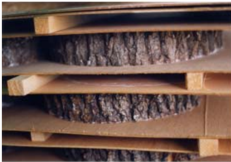
그림 4-174. A photo of oak disks stacked with pallet-type stickers made of 3mm thick plywoods.
