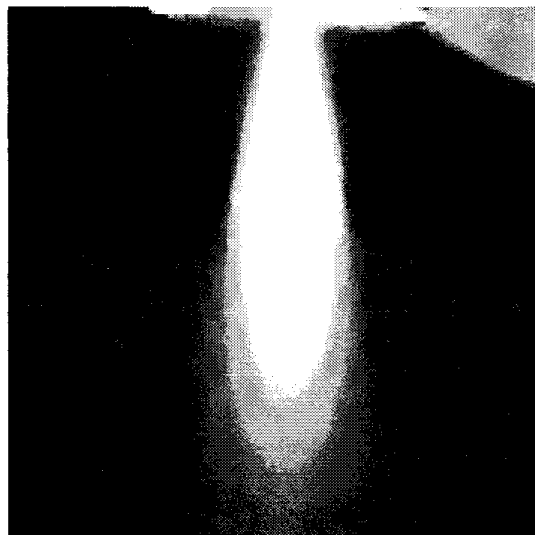
Fig. 114. Photograph of atomization column phenomenon with ultrasonic waves in tube.
