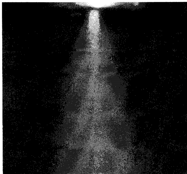
Fig. 111. Atomization phenomenon with ultrasonic waves in tube.
