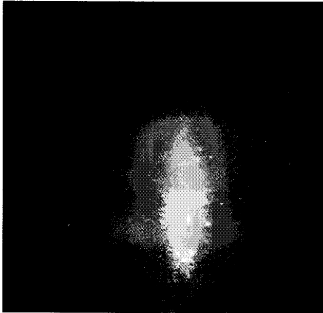
Fig. 116. Shape of droplet clusters without ultrasonic waves.
