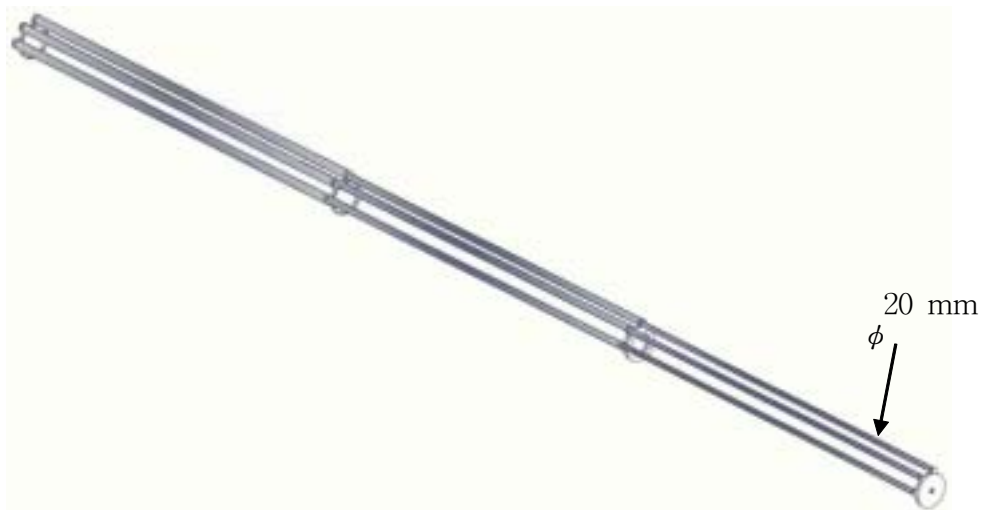
Fig 26. Assembly of supporting bar of the detachment locating hydrostatic cylinder.
