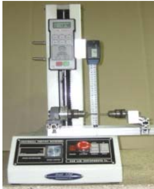
Fig 6. Torsional rigidity experiment apparatus for jujube branch.
