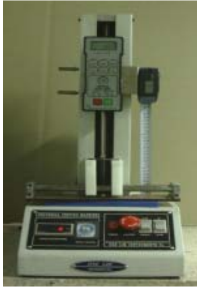
Fig 4. Elastic modulus experiment apparatus for jujube branch.
