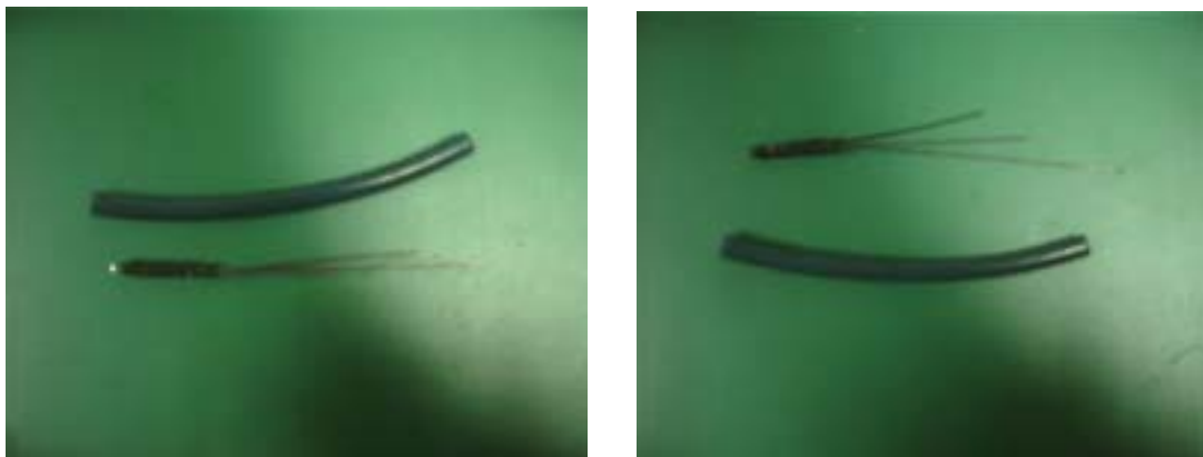
Fig 18. Urethane hose and assembly of stainless wires used as detachment rod.
