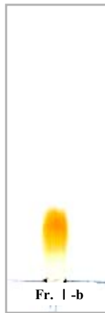
Fig. 11. Thin layer chromatogram of compound isolated from Fr I -b. developing solvent, BuOH : Acetic acid : H 2 O = 4 : 1 : 1
