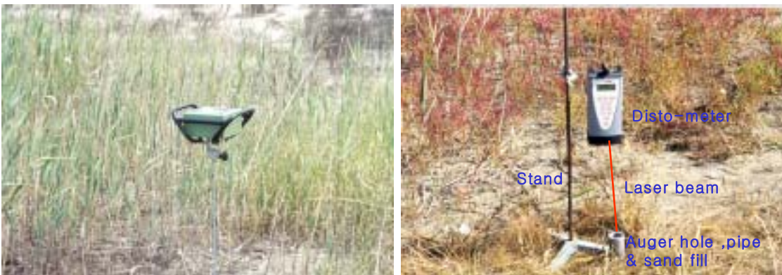
Fig. 3-1. Measurement of soil physics by penetrometer and sand-fill auger hole method.
