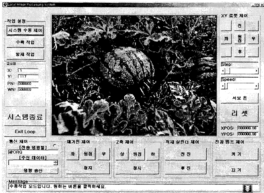
Fig. 3-4-32 Main program practice screen of the 1st prototype (touch pad screen).
