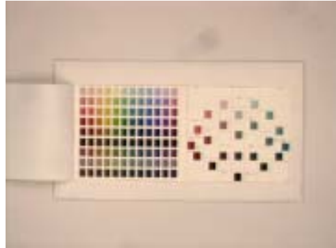
Fig. 3.3 Photo of representative color charts for white balance of RGB camera
