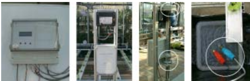
Fig. 5.11 House monitor and sensors in greenhouse II
