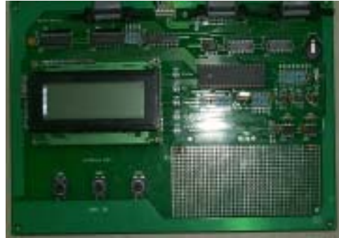
Fig. 2.16 Digital part of the house monitor
