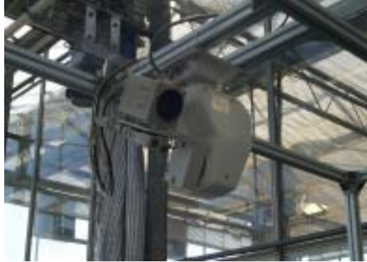
Fig. 2.7 Photograph of the internal monitoring camera & Pan/Tilt driver
