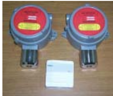
Fig. 2.4 Photograph of the Gas Sensor(SO 2 ,NO 2 ,CO 2 )
