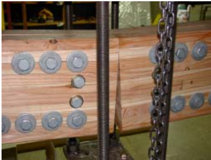
Figure 2-37. Failure of glulam beam with bolt-joint at center.
