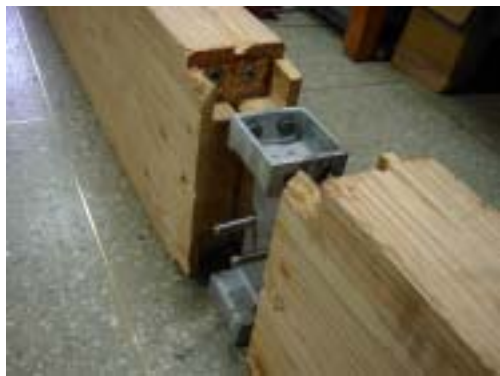
b) Shape of R-type connector
