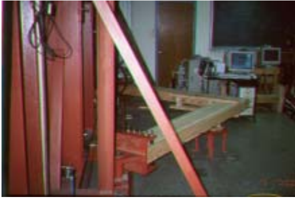
a) Testing set-up for moment-resistance of column-beam joint.
