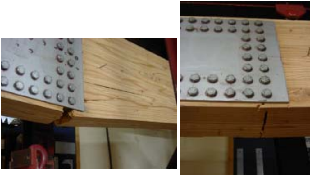
a) Failure of wood along the bolt line at GP-type joint
