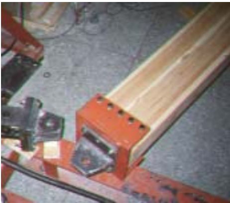
b) Connection to moving head of testing machine
