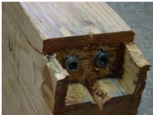
c) Withdrawal of double bolt inserted into glulam member
