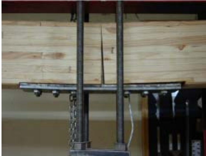
Figure 2-40. Failure of glulam beam with glued-in rod joint at center.
