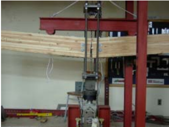
Figure 2-38. Failure of glulam beam with lag-screw joint at center.
