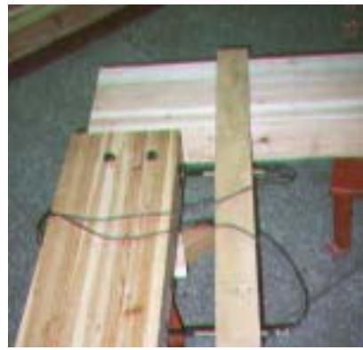
b) Attachment of LVDT to reinforced hanger joint
