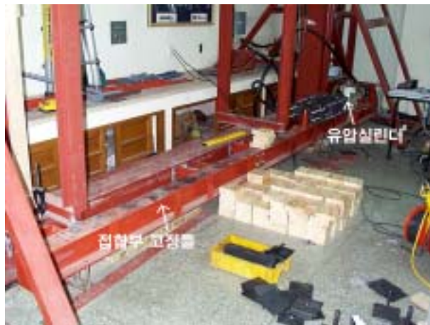
Figure 2-7. Picture of moment-resistance testing frame for glulam.
