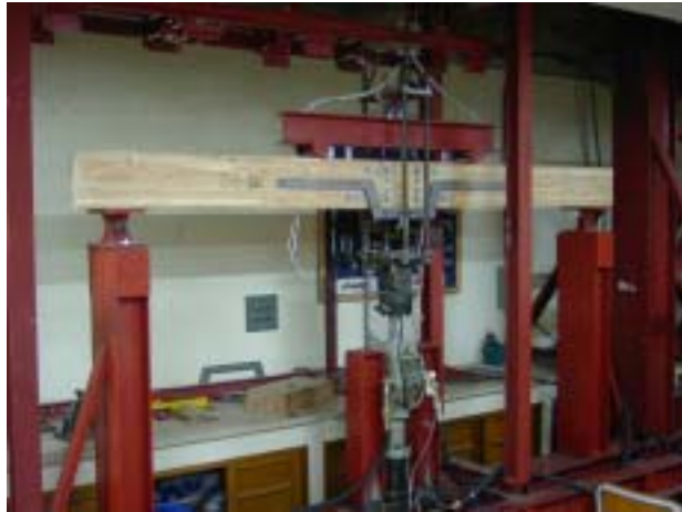
Figure 2-34. Bending test of bolt-jointed glulam beam.
