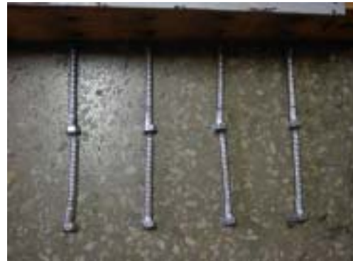
c) Deformation of lag-screw installed on bottom side
