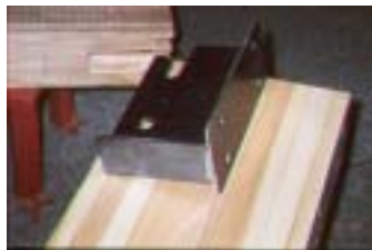
d) Picture of reinforced hanger connector
