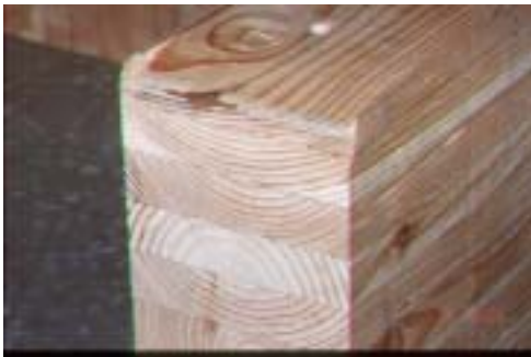
a) Deformation perpendicular to grain under steel plate
