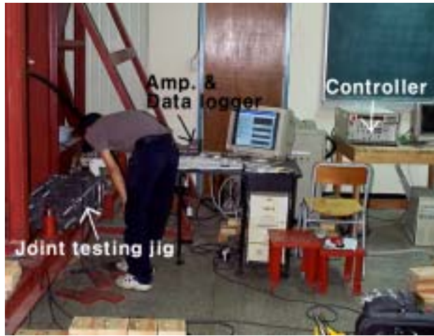
Figure 2-5. Overall testing arrangement for bolted joints.
