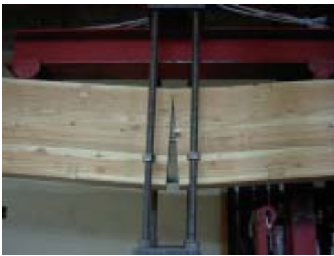
a) Widening of gap between members within SCP-type joint
