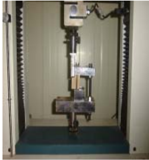
Fig 2. Apparatus of shearing test
