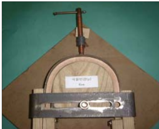
Fig 1. Apparatus for bending process
