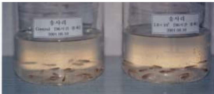
Fig. 73. Toxicity test of Penicillium sp. PS-113 conidia (inoculum : 1.0 \times 10^8 conidia/ml) against monnow ( Oryzias latipes ), a kind of fish, during 96 hours treatment.
