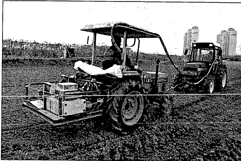
Fig. 5-8 Scheme of motion resistance test.
