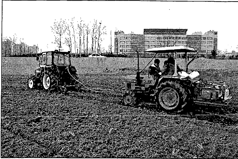
Fig. 5-7 Scheme of drawbar pull test.
