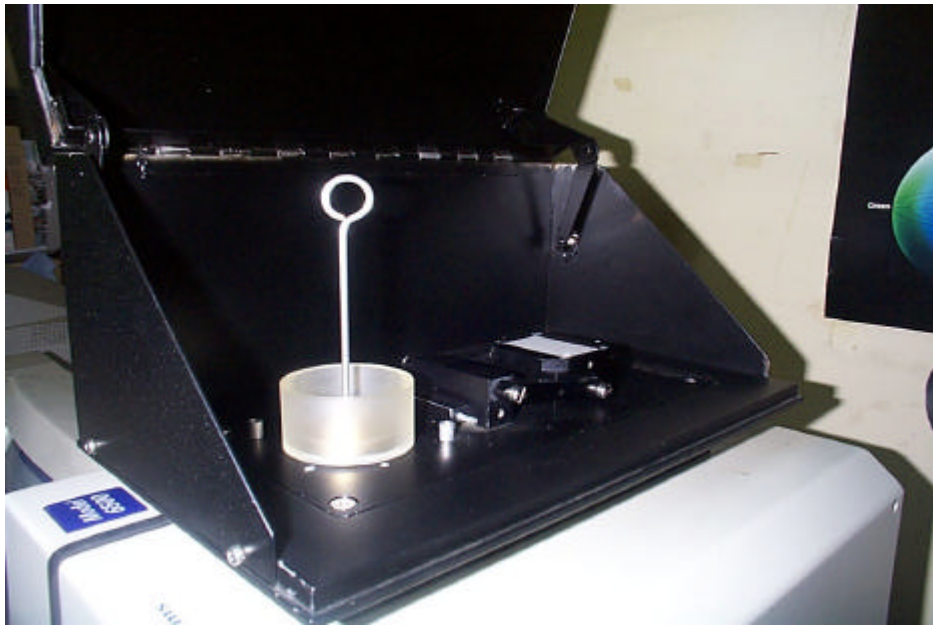
Figure 3-2. Spectrophotometer and horizontal module for reflectance spectrum measurement
