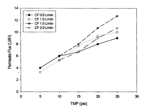
그림 28. Permeate flux with TMP as a function of retentate flow rate during ultrafiltration
