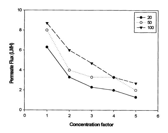
그림 29. Permeate flux as a function of concentration factor with various solvent-feed ratio during ultrafiltration
