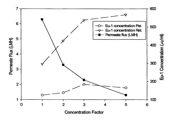
그림 30. Eu-1 concentration and permeate flux as a function of concentration factor during ultrafiltration
