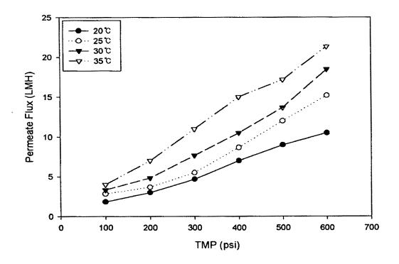
그림 31. Permeate flux as a function of TMP with various temperature during reverse osmosis
