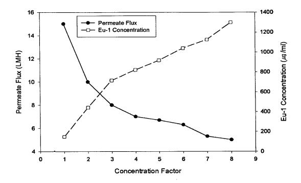
그림 32. Eu-1 concentration and permeate flux as a function of concentration factor during reverse osmosis
