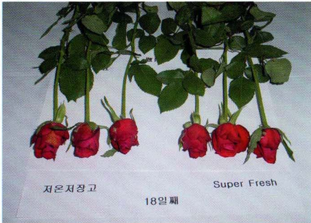
Fig.47. Visual quality of roses after 18 days storage at 5°C conventional and super fresh cooler attached cold room.
