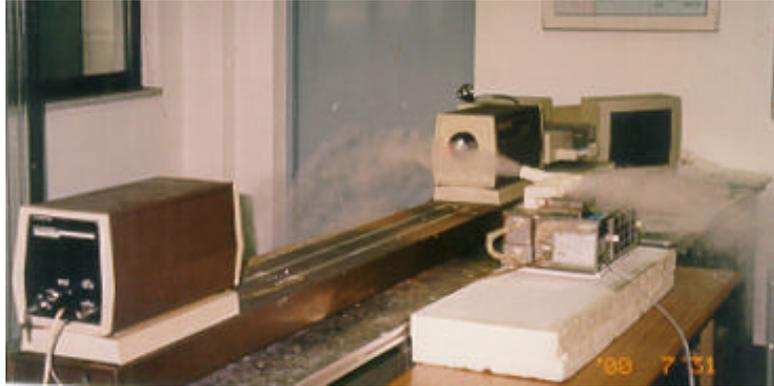
31. Laser diffraction particle size 가
