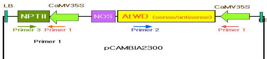
Figure 39. Construction of Atwd sense/ antisense plant expression vector
