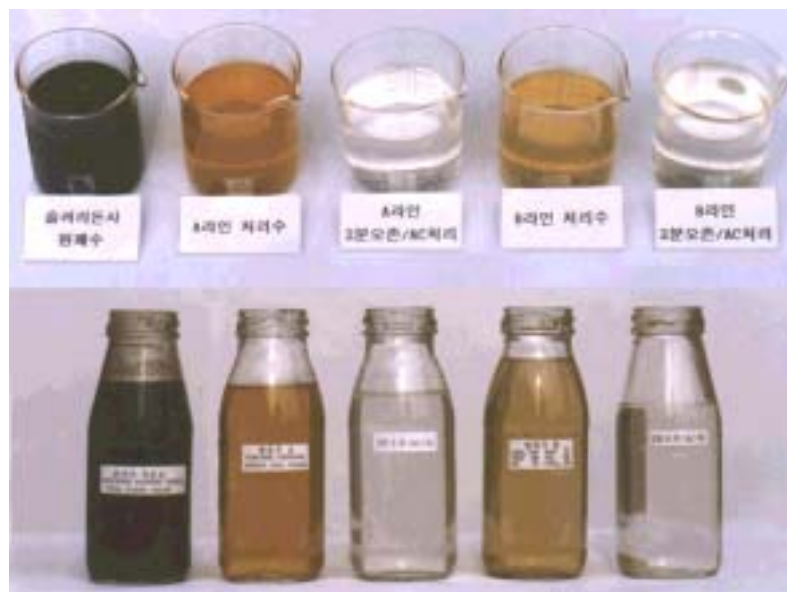
photo.39 Color comparison of Ozone and activated carbon at effluent
