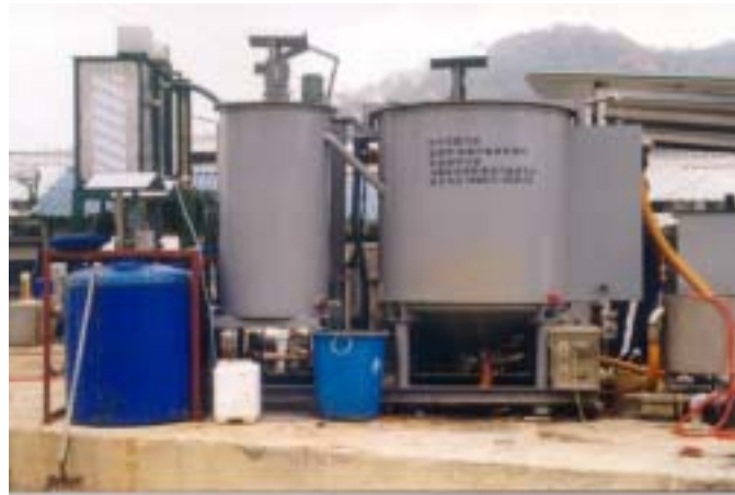
photo.19 Solid/liquid separation system of round type
