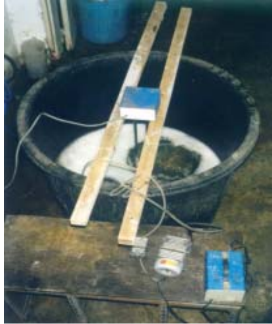
photo.25 Ammonia stripping picture
