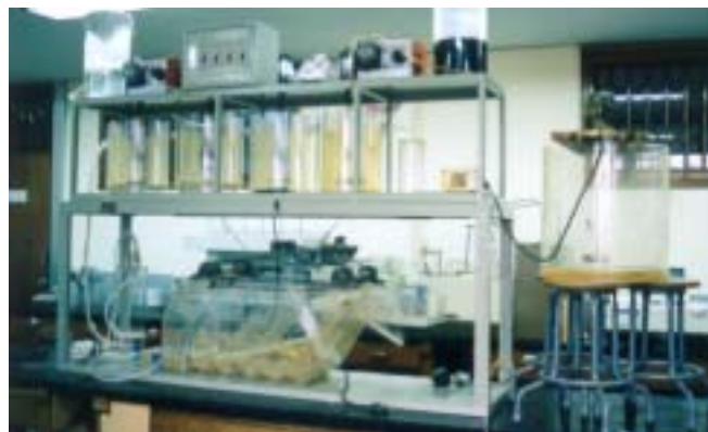
photo.5 Coagulation tank and flotation separation reactor used for experiment
