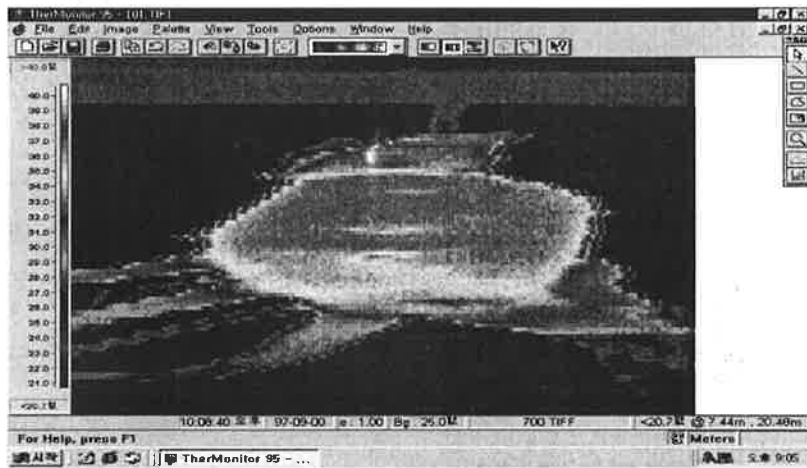
Fig 2-11 Temperature distribution of fresh ginseng heated in an oven.
