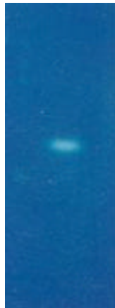
Fig. 4-3. TLC chromatogram of standard vomitoxin. (Developing solvent=toluene: acetone: methanol=5:3:2,v/v)
