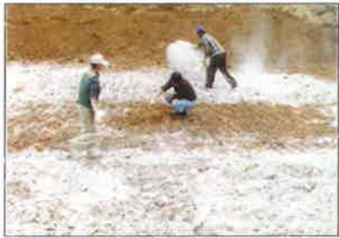
Photo 3. Gypsum treatment in planting foundation and improvement experiment site.
