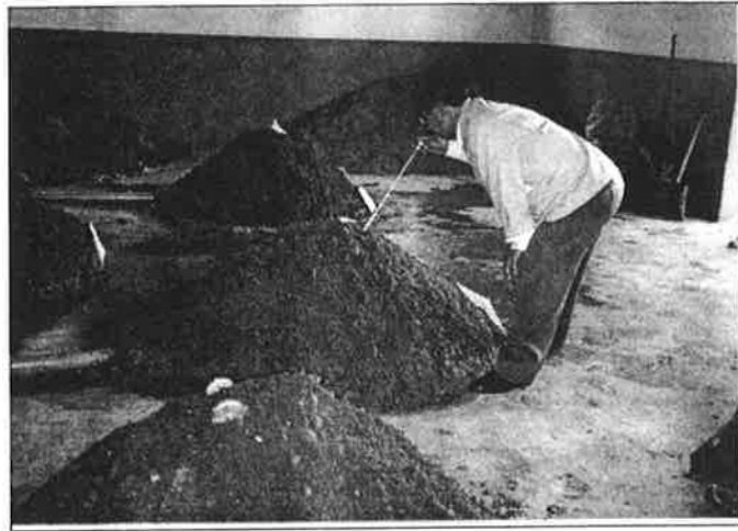
Photo 3-1. Composting by pile and blow method
