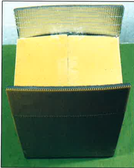
Fig. 7. Cooling box made of plastic corrugated board
