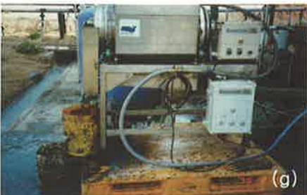
(g) Cyclone Drum Filter
