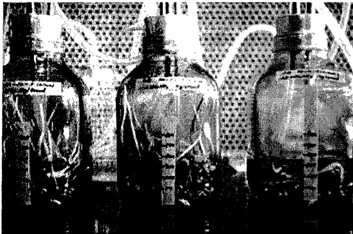
Fig. 7. Configuration of 500 mL carboy for nitrogen concentration test.
