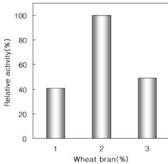
Fig. 2-7. Effect of wheat bran concentration on the production of xylanases by S. thermocyaneoviolaceus at jar-fermentor incubation. The culture conditions were the same as Fig. 2-5 except basal medium which was composed of 0.06% yeast extract, 0.06% bactopectone, 0.05% MgSO_4 \cdot 7H_2O , 0.005% FeSO_4 \cdot 7H_2O , 0.05% KH_2PO_4 and 0.2% K_2HPO_4 (pH 7.0).
