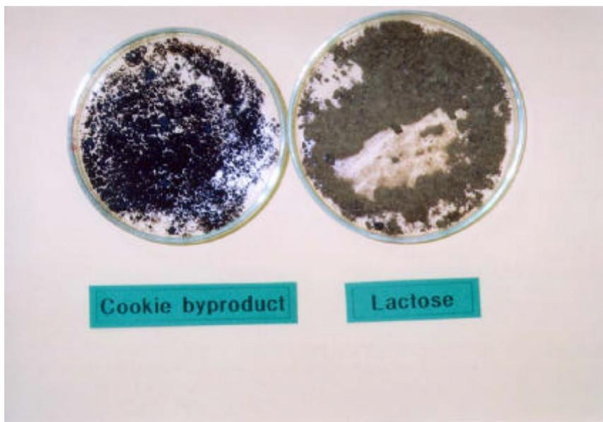
Fig. 2-21. Photograph of morphology of lactose compared with cookie byproduct after heat treatment
