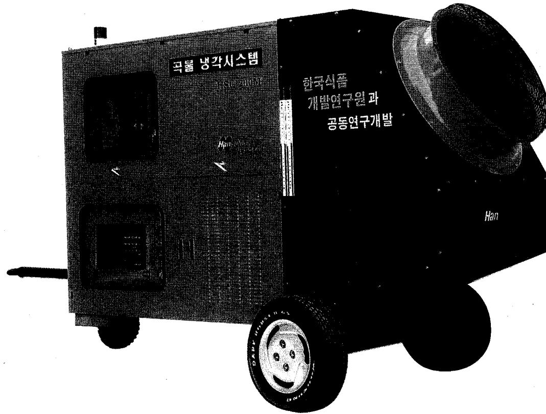
Fig. 4-10 Photograph of the prototype grain cooler(HSC-200M).
