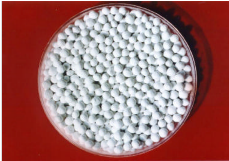
Photo 14. Picture of smooth surface of pellet seed with PS
