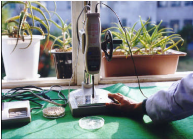
Photo 16. Picture hardness testing of pellet seed
