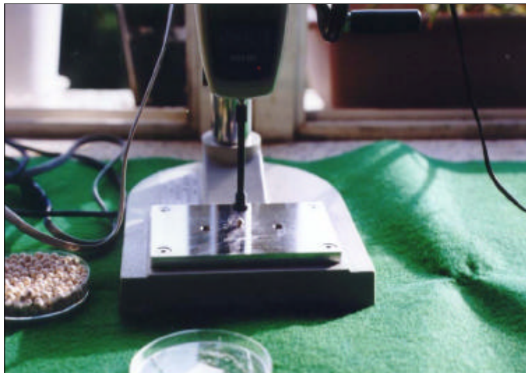
Photo 17. Picture hardness testing of pellet seed
