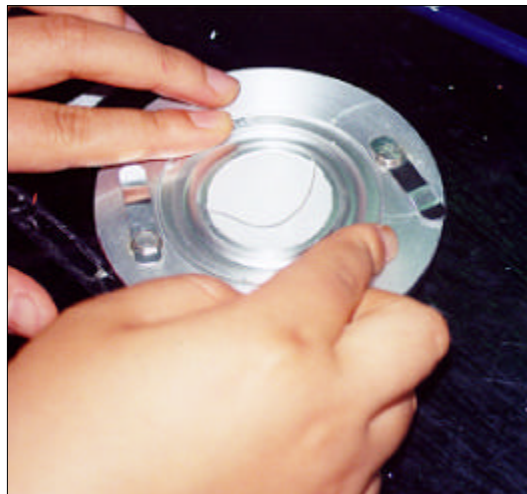
Fig. 3.1. Schematic diagram(a) and photograph(b) for measuring NIR spectrum of liquid sample using the aluminium cell.
