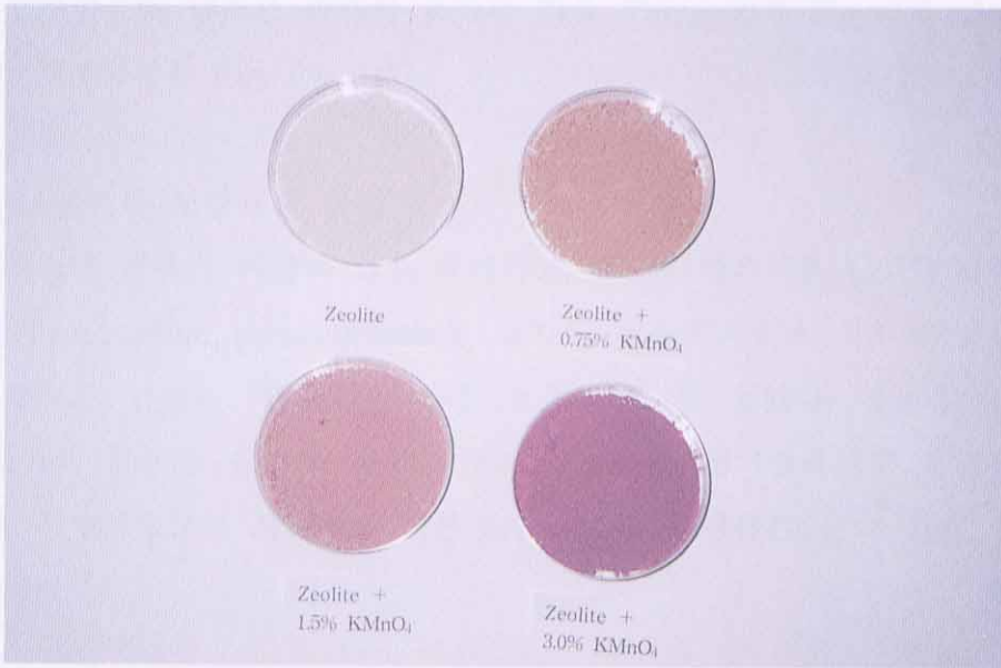
Fig. 2. Additive materials used to modify a polyethylene film
