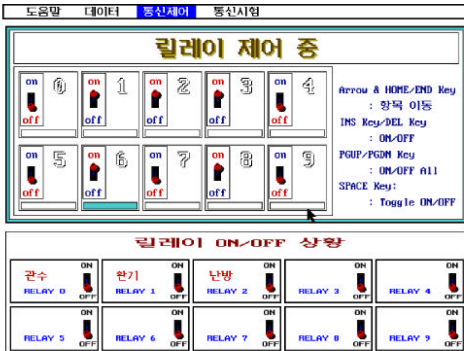
Fig. 6-27 The screen display at monitoring computer showing the remote changing of
