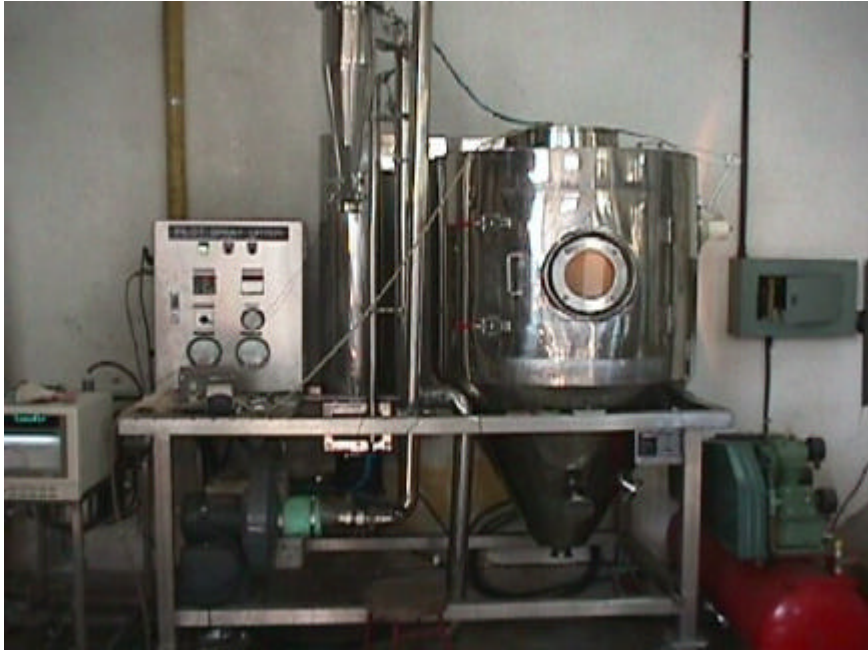
Fig. 2-1. The experimental set for Spray drying of soy milk
