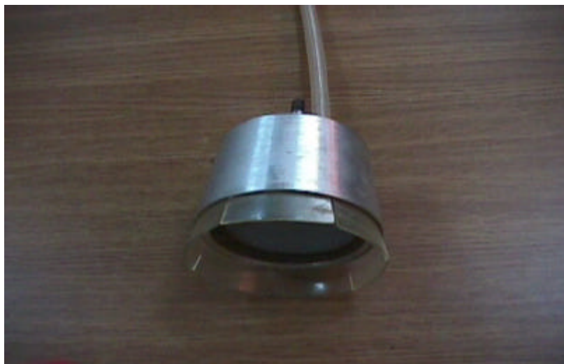
(b) The assembled upper molding frame
