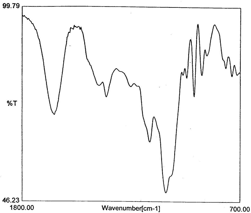
Fig. 22. FT-IR spectrum of agar purified with propanol.
