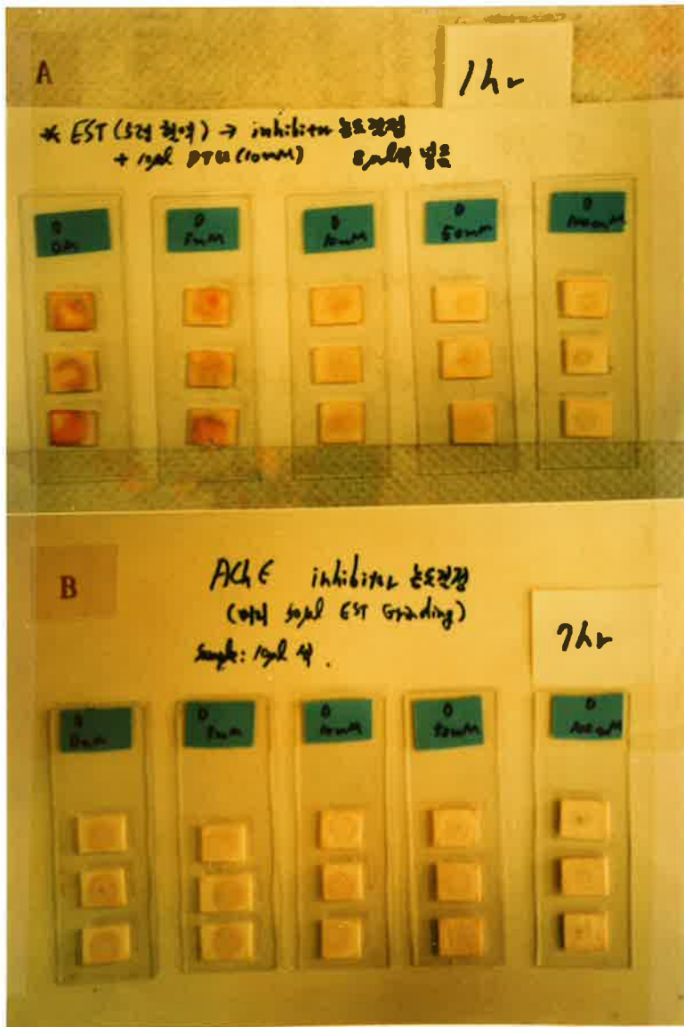
Fig. 5. Examples for determining diagnostic insecticide concentrations in esterase (A) and acetylcholinesterase (B) diagnostic kits
