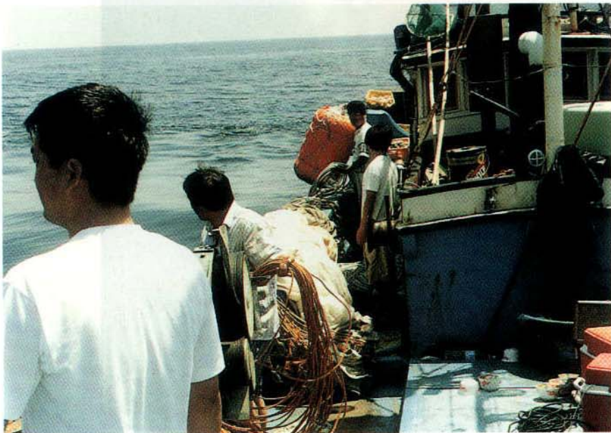
Photo. 2-4. Manual anchoring operation of sea anchor system in a squid jigging boat of 19ton.
