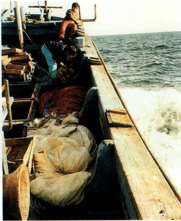
Photo. 2-3. Sea anchor system ready for manual anchoring operation.
