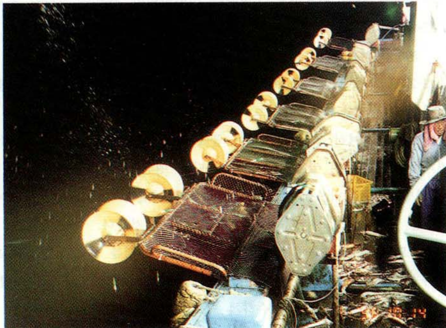
Photo. 2-2. Squid jigging operation by automatic jigging machine.
