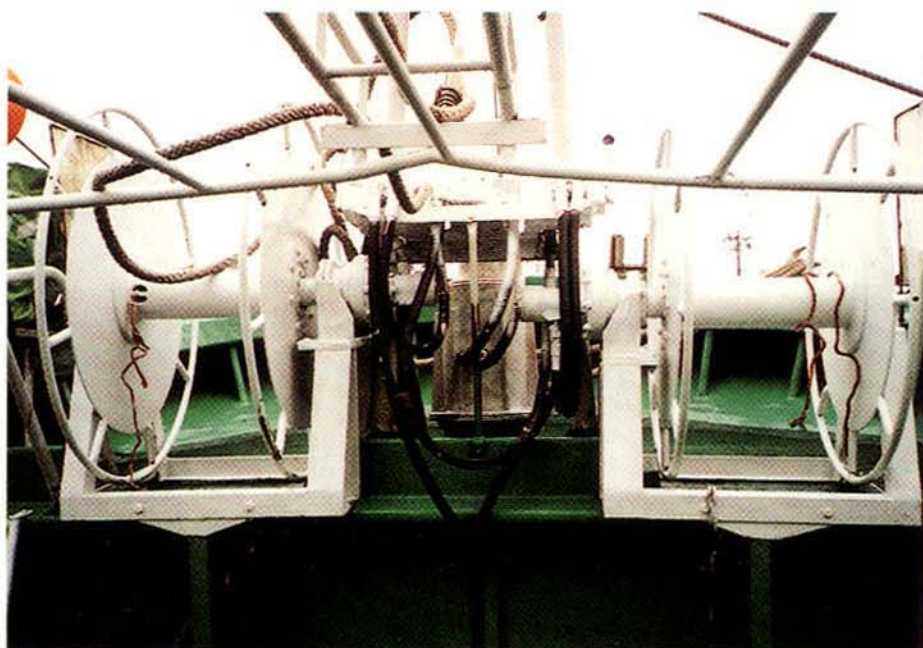
Photo. 2-10. Hauling machine of sea anchor system with twine drum in Japan.
