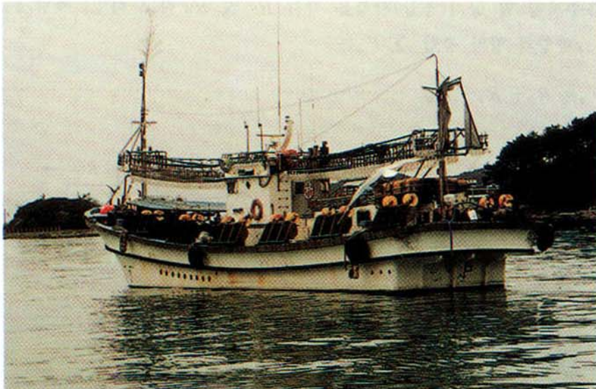
Photo. 3-3. Commerical squid jigging boat 95 Gillyang-Ho(29ton) used for the experiment.
