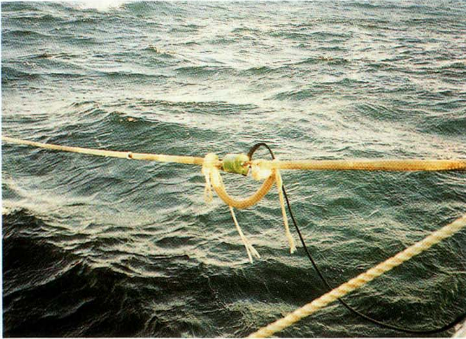
Photo 3-2. Wind and wave monitor system (a) Load cell
