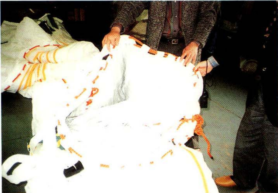
Photo. 2-8. Vent part of sea anchor.
