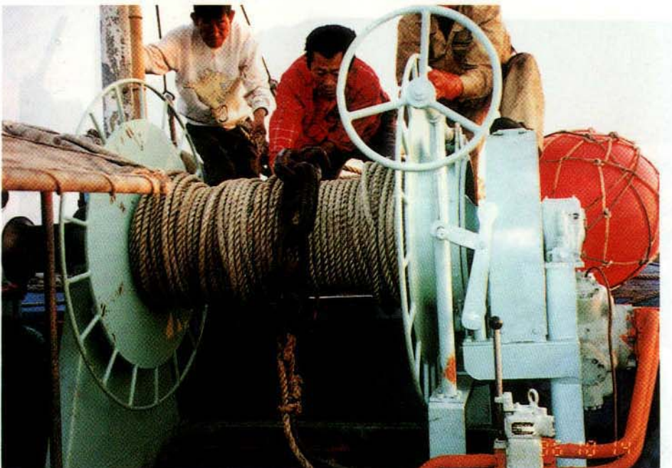
(b) Unpacking operation of the sea anchor system to pick out sinker
