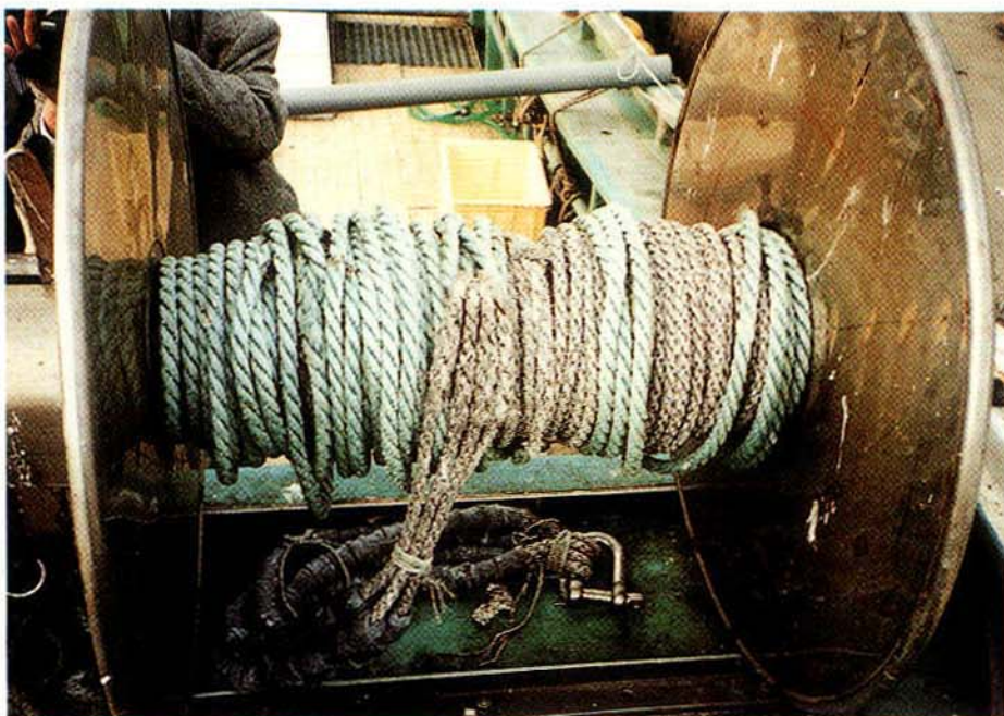
Photo. 2-9. Hauling machine of sea anchor system with single side drum in Japan.
