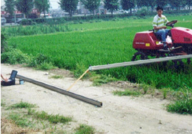
Fig 10- 8. A system of boom tip behavior measurement
