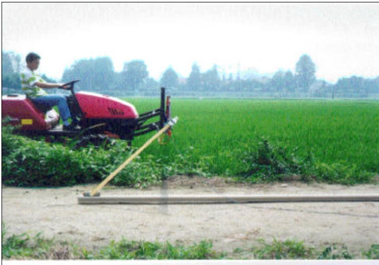
Fig. 10- 7. Side view of boom tip behavior measurement system
