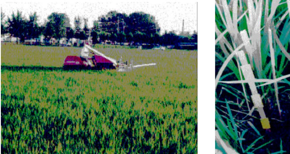
Fig. 11-2. Coverage rate test and sensitive paper arrangement of boom sprayer
