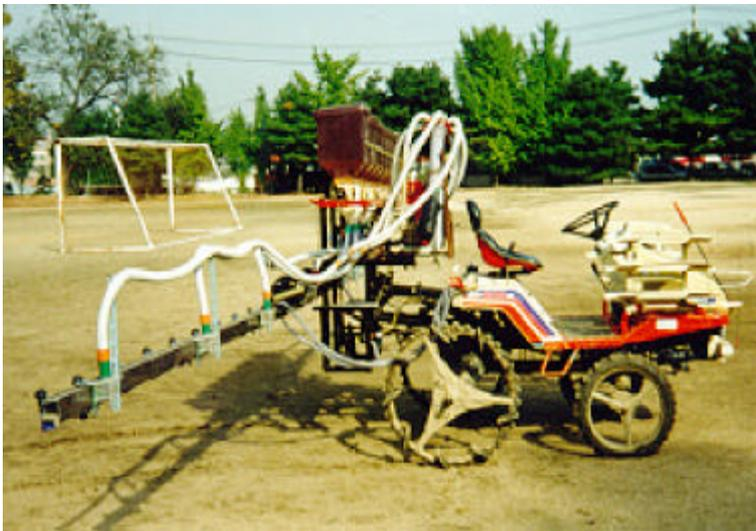
Figure 7-12. Feature of applicator attached in transplanter
