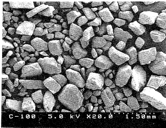
Fig. 9. Scanning electron micrographs of CAP-coated limestone granule
